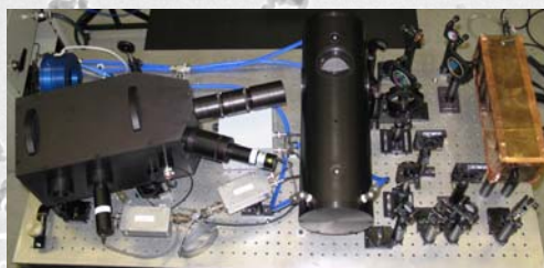
Optical layout of first generation high sensitivity system HS-LII-1
