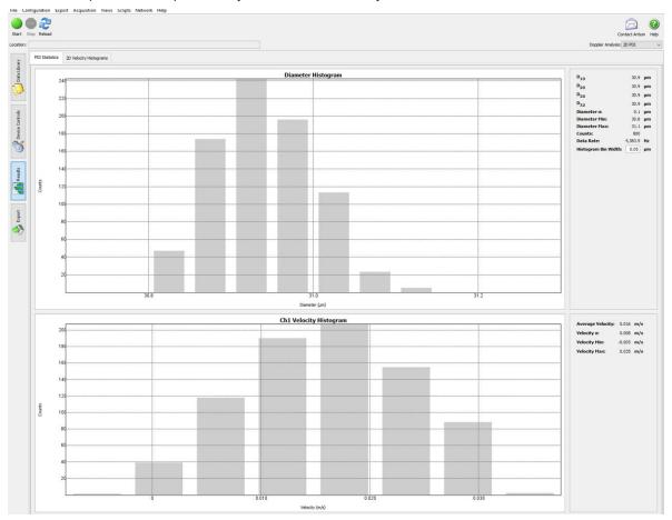
Droplet size and velocity distributions collected while scanning across a multiple-nozzle inkjet printhead. Drop size standard deviation across all nozzles less than 0.1 µm.
