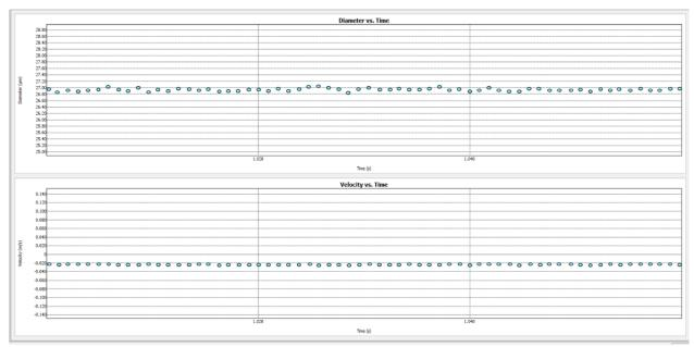
Time history for droplet diameter and velocity produced by an inkjet printer.
