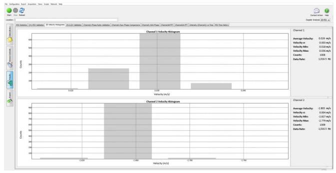
Two components of droplet velocity measured with stability of 3 to 4 mm/s and a resolution of 1 mm/s.
